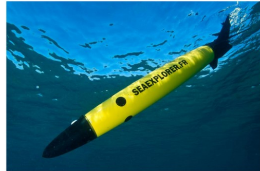
(d) Underwater Gliders Power availability: ultra-low Telemetry: satellite (intermittent)
