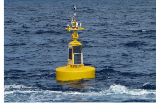
(b) Moored Buoys Power availability: Medium Telemetry: GSM / satellite
