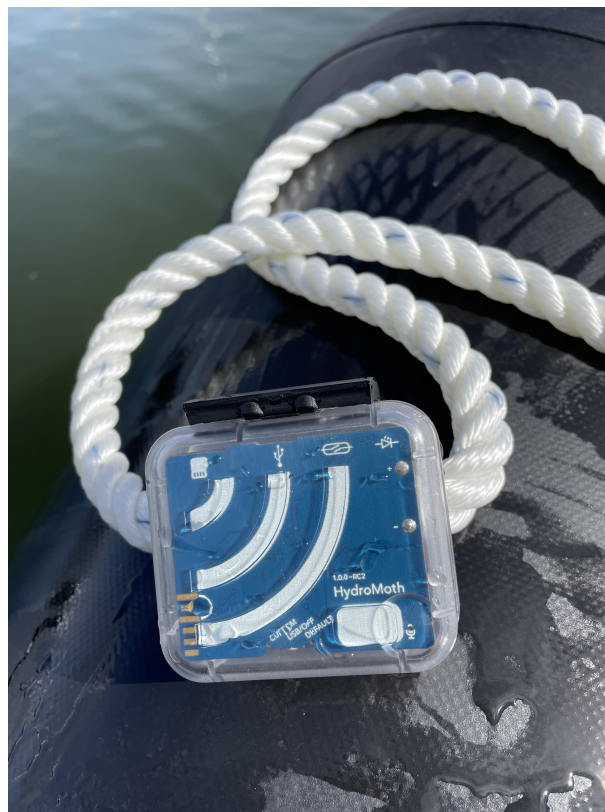
Figure 5: HydroMoth cable-tied to a weighted line prior to deployment from a small boat.
